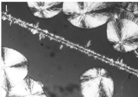
**Figure 3.** Shear-induced transcrystallization of PP in glass fiber/PP composites, showing the appearance of  $\alpha$ -crystalline modification of iPP on the fiber's surface (polarizing optical micrograph of a single glass fiber after partial melting of the matrix) [59]
